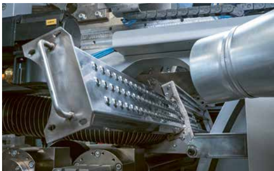
Optimized configuration creates homogenous heat transfer and improves drying capacity
